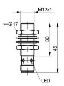
**Inductive Sensors** BES 516-329-E5-C-S 4 M12x1 x 45 normally-open Sn=2mm shielded
